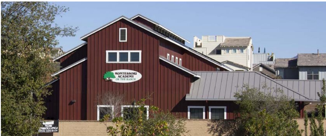
Variety in roof forms and ridge heights, layering of eaves and the introduction of single story elements break up the mass of the individual buildings and create a varied skyline.
